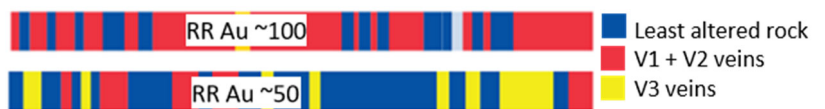
Examples of different amounts of veins, vein types and host rock in two intervals (each 10 m long) from a gold deposit. Upper interval (RR Au = 100) has more abundant V1 and V2 veins and less least altered rock than the interval with a lower RR Au.
